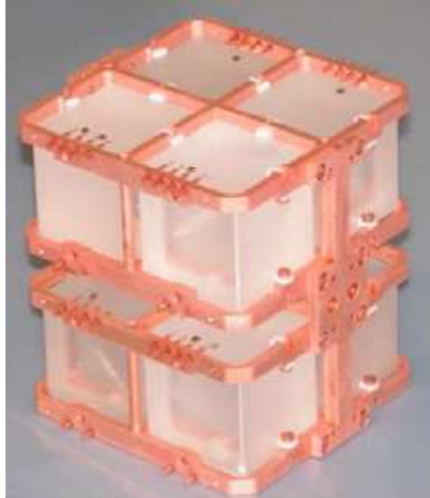
Figure 3.3: The basic RAD detector, used in the R&D activity of the CUORE collaboration focused on background investigation.
