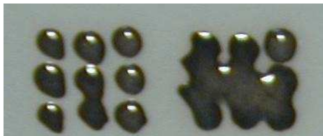
Figure 6.8: An example of the effect of high humidity in the gluing environment: black epoxy spots.
