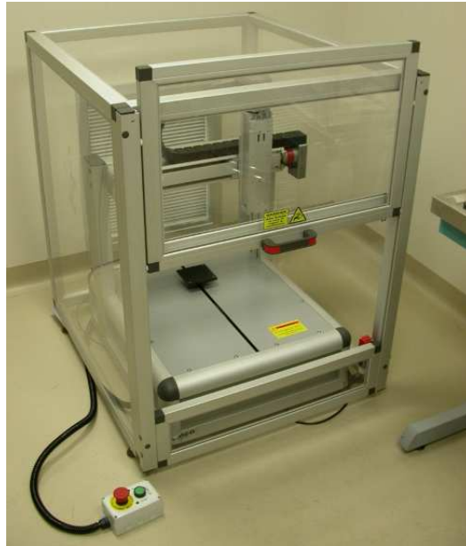
Figure 6.15: The table-top cartesian robot WR300 used in Como dispensing tests.
