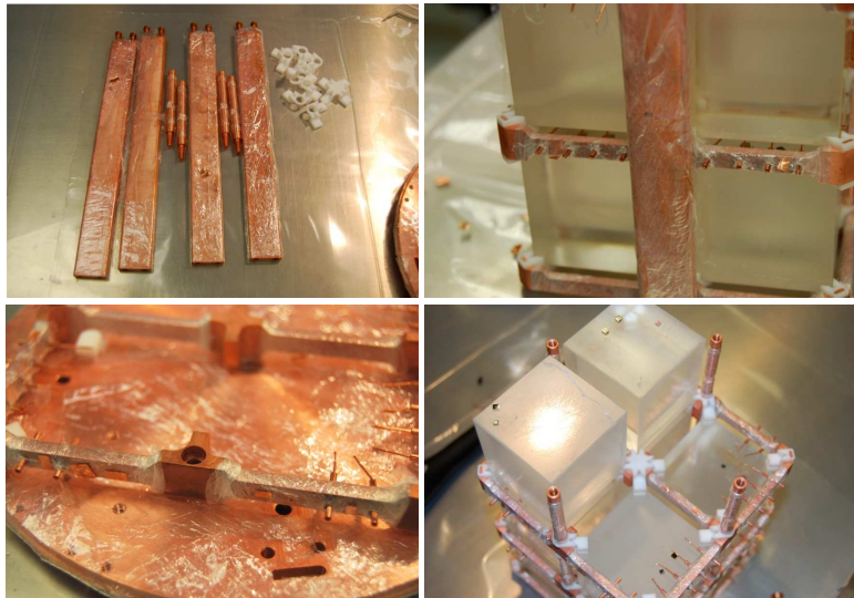
Figure 3.9: The RAD-Polyethylene treatment for Cu surface processing: coverage of the holding structure with polyethylene layers.
