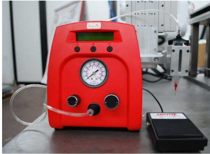
Figure 6.20: The pneumatic Loctite 98666 epoxy dispenser.
