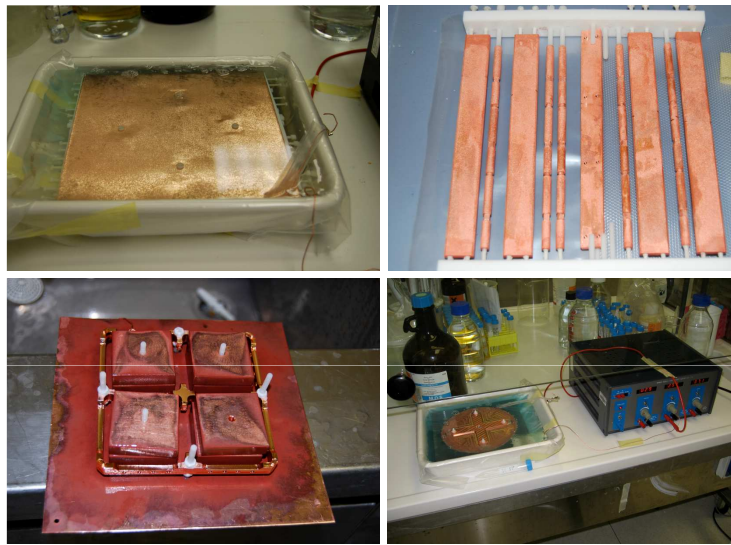
Figure 3.10: The LNGS protocol for Cu surface processing: setup for the electro-polishing of Cu columns, bars (top), frames and shielding (bottom).
