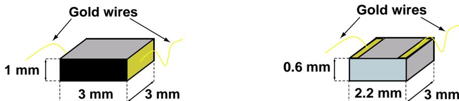
**Figure 5.5:** Different position of golden pads in the CUORICINO-like (left) and flat-pack (right) NTD thermistors. In contrast to the CUORICINO case, the flat pack option allows to bond golden wires for detector readout when the thermistors are already glued on the crystals.
