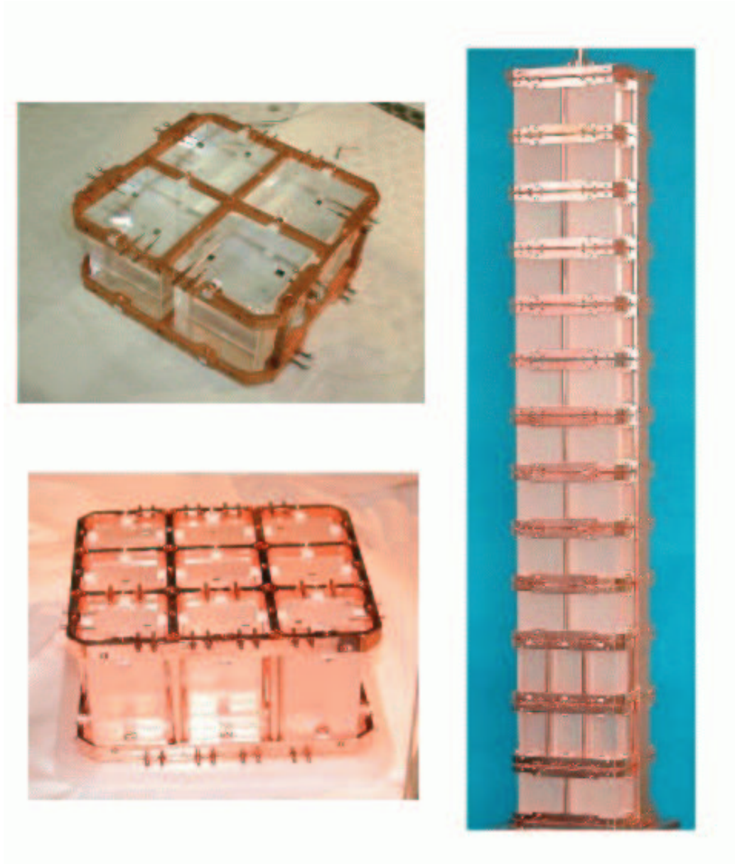
Figure 1.2: The tower of CUORICINO and the four and nine crystal modules.
