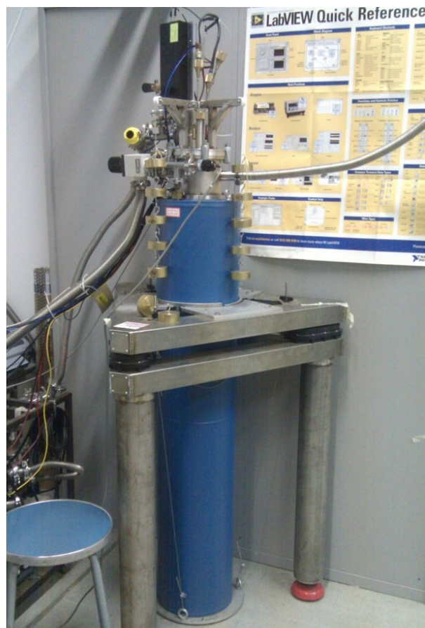
Figure 6.18: Experimental setup for the measurement of the Kevlar creep. The three capacitors are arranged inside the dewar refrigerator.
