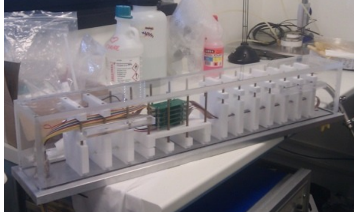
Figure 5.12: A picture of the experimental setup realized for the measure of the impedance of the CUORE-0 PEN-Cu tapes.
