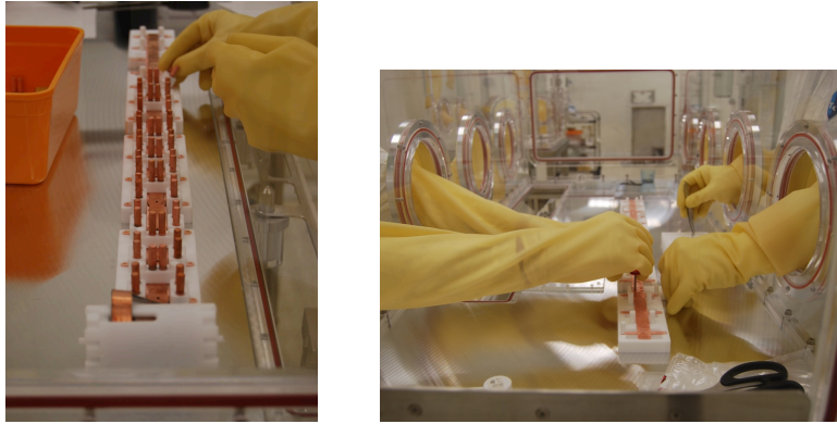
Figure 5.9: The operation of coupling of the wire tapes to the wire trays during the commissioning of the assembly line.
