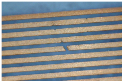
Figure 5.16: Example of a broken copper track.
