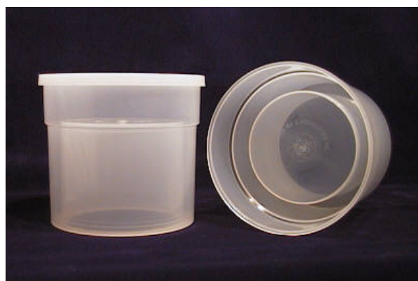
Figure 5.19: Photo of the type of Marinelli beaker used in the gamma measurements of the irradiated TeO 2 powder and the two extended sources. Photo was taken from Ref. [104].
