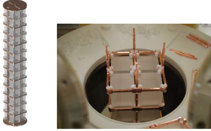
Figure 3.9: CUORE-0 tower rendering and close up. Left: the 52 \times 5 \times 5 \text{ cm}^3 \text{TeO}_2 crystals of 750 g each are set up in 13 floors in groups of 4, for a total mass of 39 kg. The tower skeleton is made of ultra-clean copper and the crystals are plugged to the frames by PTFE clamps. Right: close up of the tower during the assembly; crystals, copper structure and PTFE brackets (white components) are visible.
