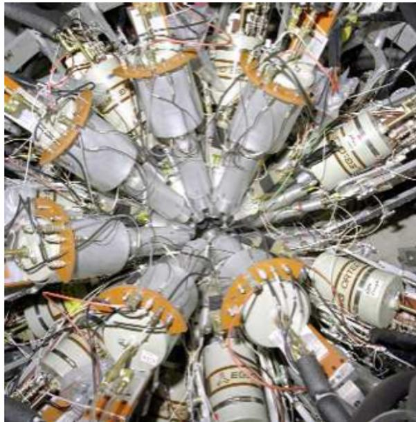
Figure 5.6. Top: Illustration of a single Compton suppressed HPGe detector. Bottom: Photograph of the GEANIE detector, with no target in place. The detector is a spherical arrangement of 26 individual HPGe detectors on the 60R beamline at LANSCE. Figures courtesy of the GEANIE collaboration.
