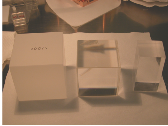
Figure 7.1: A 6 \times 6 \times 6 \text{ TeO}_2 crystal (left) compared with the old CUORICINO 5 \times 5 \times 5 and MiBeta 3 \times 3 \times 6 .
