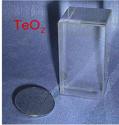
Figure 3.2 - Example of \text{TeO}_2 crystal used in the Milano group. The crystals are produced by Shanghai Institute of Ceramics (Shanghai, China).
