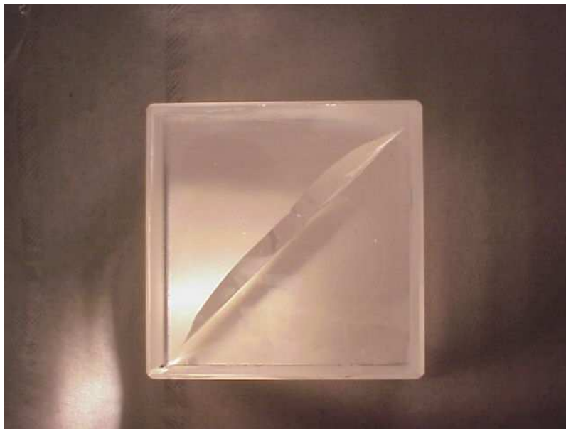
Figure 5.6 - Picture of a polished crystal. It is possible to see the big internal fracture.
