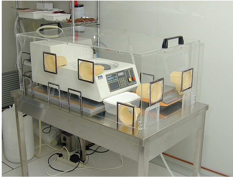
Figure 5.11 - Picture of the anti-radon box placed in the white room of Hall A at LNGS. The silicon tubes flux pure nitrogen in the chamber.
