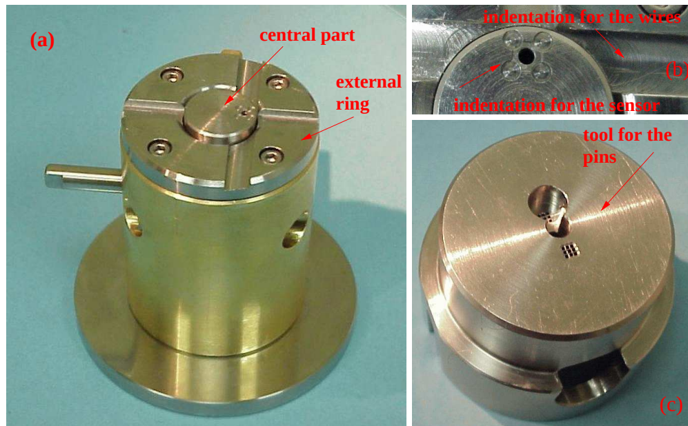
Figure 5.19 - The tool used in the MiDBD experiment to attach the sensor to the energy absorber with glue spots.
