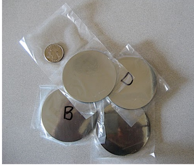
Figure 3.2: Germanium wafers used to make NTD Ge thermistors.
